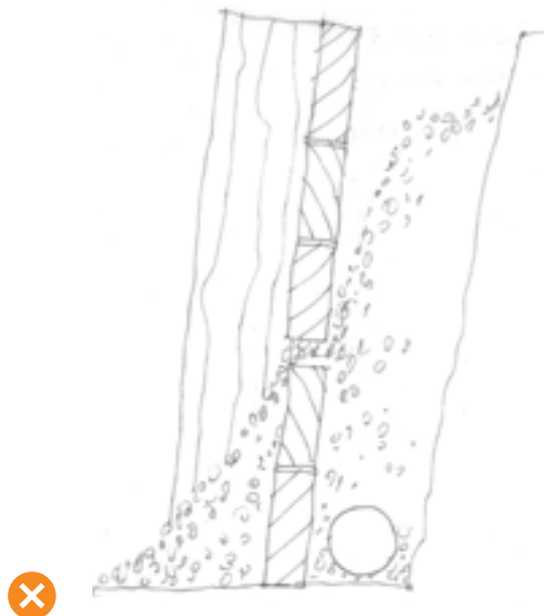
Figure 4 Coarse fill passing through a timber retaining wall.
